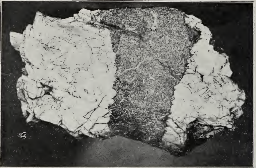
FIG. 8. Coarsely crystalline, white vein calcite separated by irregular stylolitic partings from gray limestone. The replacement of limestone by calcite was checked by the relatively insoluble materials of the stylolitic bands. About one-third natural size. Cullen Mine, near Salem, Kentucky.
